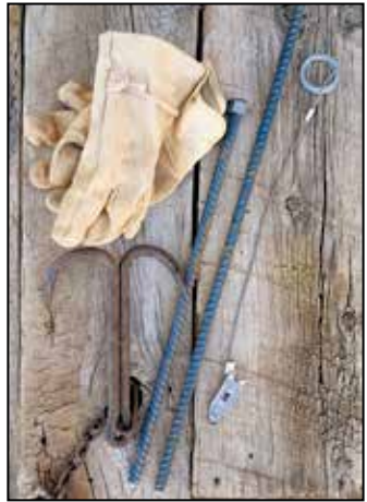
Left to right: Drag, 18" stake, 24" stake and earth anchor (disposable type). NMDGF photo.
